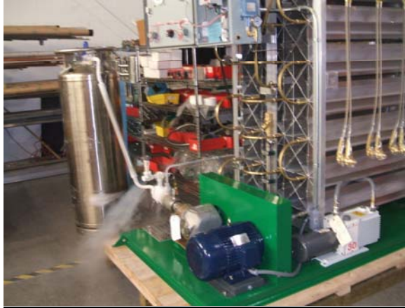
PPS 10K: 10,000 SCFH/LOX/LIN/LAR PORTABLE PUMPING STATION COMPLIES WITH ALL PRAX GS STANDARDS
